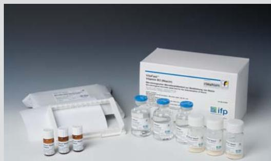
The VitaFast® test kit contains a microtiter plate coated with micro-organisms (96 wells), an additional holder, three adhesive foils, three bottles assay-medium, three standard bottles and three bottles sterilized water.
